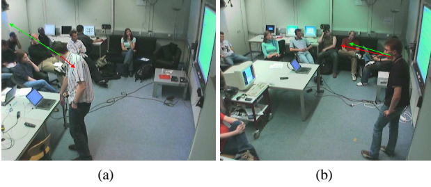
Fig. 4. Images from two experimental cases. In (a), speaker is bowing his head towards the laptop and video based head orientation estimation does not produce an accurate result (red vector) while audio estimation (green vector) generates a more accurate output. Estimation reliability is proportional to vector length. In (b), an example where both estimators outputs a correct result.
